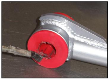
3. Generously grease the outer diameter of the supplied TC metal inner sleeves.
