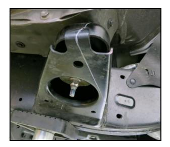
2. After the body mount is cut, make a template (or order Total Chaos part number 59850) then box in the body mount.
