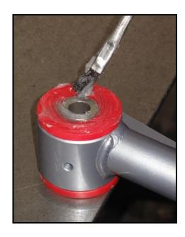
6. When installing the zerk fittings, it may be necessary to use a knife or sharp object to clean out the top of the threaded hole so the ½"-28 NTP threads will catch. When tightening the zerk, <u>DO</u>
