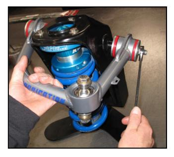
3. With the bolt loose, pump grease into the zerk fitting until you can see the excess grease bleed out from between the bushing "hat" and the plated end washer.
